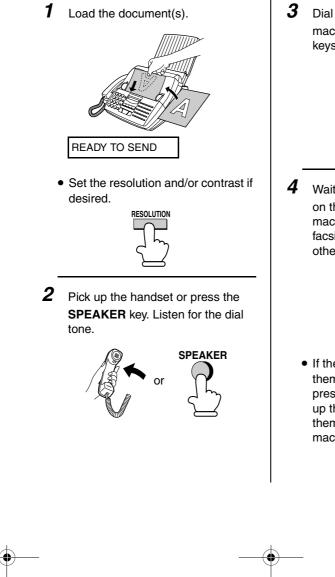
Dial the number of the receiving machine by pressing the number keys.
